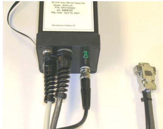
Figure 16 - Cabling of AR4000 with 200 KHz capability
